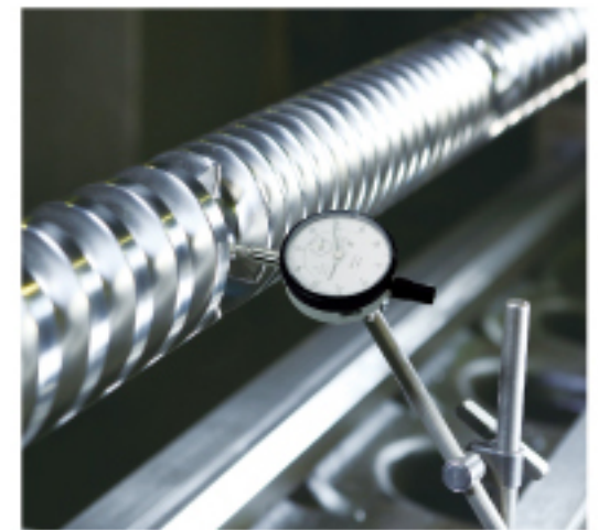
Screw straightness test / 螺桿真直度測量
