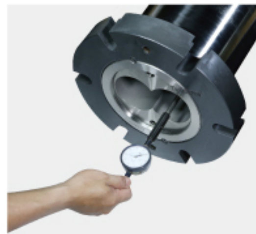
Hardness of a twin-barrel test 雙直孔套筒內孔硬度測量
