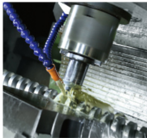
Finishing of the screw flights on a CNC thread milling machine / CNC螺桿加工機加工牙型
