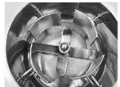
MB Type Inner Plate Water Guiding to Enlarge Cooling Area. (Standard)
